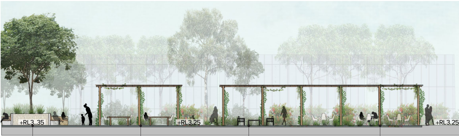
Raised Planter with timber batten seating edge Dining table seating Lounge seating Timber frame pergola with climbers planted to columns Section through Garden Rooms next to Village Green
